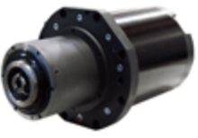
ES883 Kw 19-S1/22,8-S6 - HSK E63 - 24,8Nm S1 - long nose - 15.000rpm - liquid 380V - *cables connector
