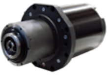
ES883 Kw 29,3-S1/35,2-S6 - HSK E63 - 28,6Nm S1 - long nose - 15.000rpm - liquid 380V - *free cables
