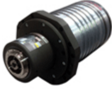
ES798 - H6161H1110 Kw 22,0-S1/25,0-S6 - HSK A63 - 28Nm S1 - 20.000rpm - liquid cooling 350V - encoder LB 1Vpp
