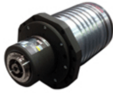
ES798 - H6161H1134 Kw 22,0-S1/25,0-S6 - HSK A63 - 28Nm S1 - 20.000rpm - liquid cooling 350V - encoder LB 1Vpp - Rotary Joint
