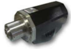
ES798 - H6161H1147 Kw 22,0-S1/25,0-S6 - HSK A63 - 28Nm S1 - 20.000rpm - liquid cooling 350V - encoder LB 1Vpp
