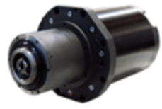
ES883 Kw 29,3-S1/35,2-S6 - HSK E63 - 28,6Nm S1 - long nose - 15.000rpm - liquid 380V - *cables connector
